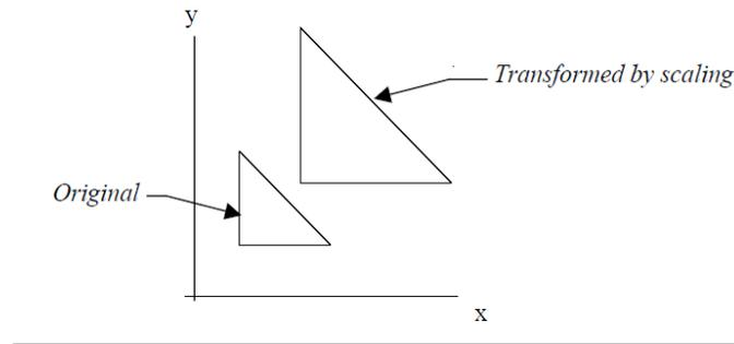
Note that the new coordinates represent the original value times the scale factor. The old and the new positions of the triangle are shown in the figure above.
