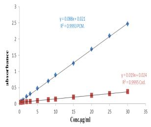
Fig. 2: Calibration curves of PCM and COD in mixture.
