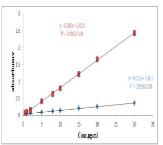
Fig. 3: Calibration curves of PCM and COD alone.
