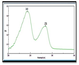
Fig. 1: UV – Spectrum of Paracetamol and codeine mixture.
