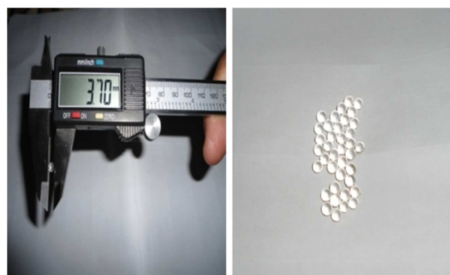
Figure 1. Vernier calliper used for measuring the diameter of gel bead.
