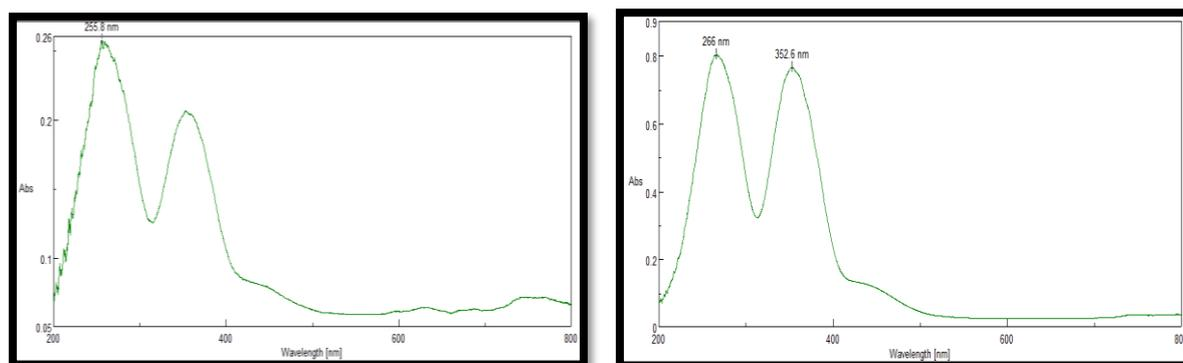
**Fig. 2: Potassium dichromate and Sodium nitro prusside solution spectra.**
